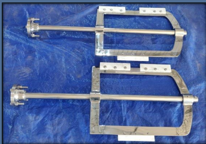
Anchor Agitator Assembly (Pharma Application)
