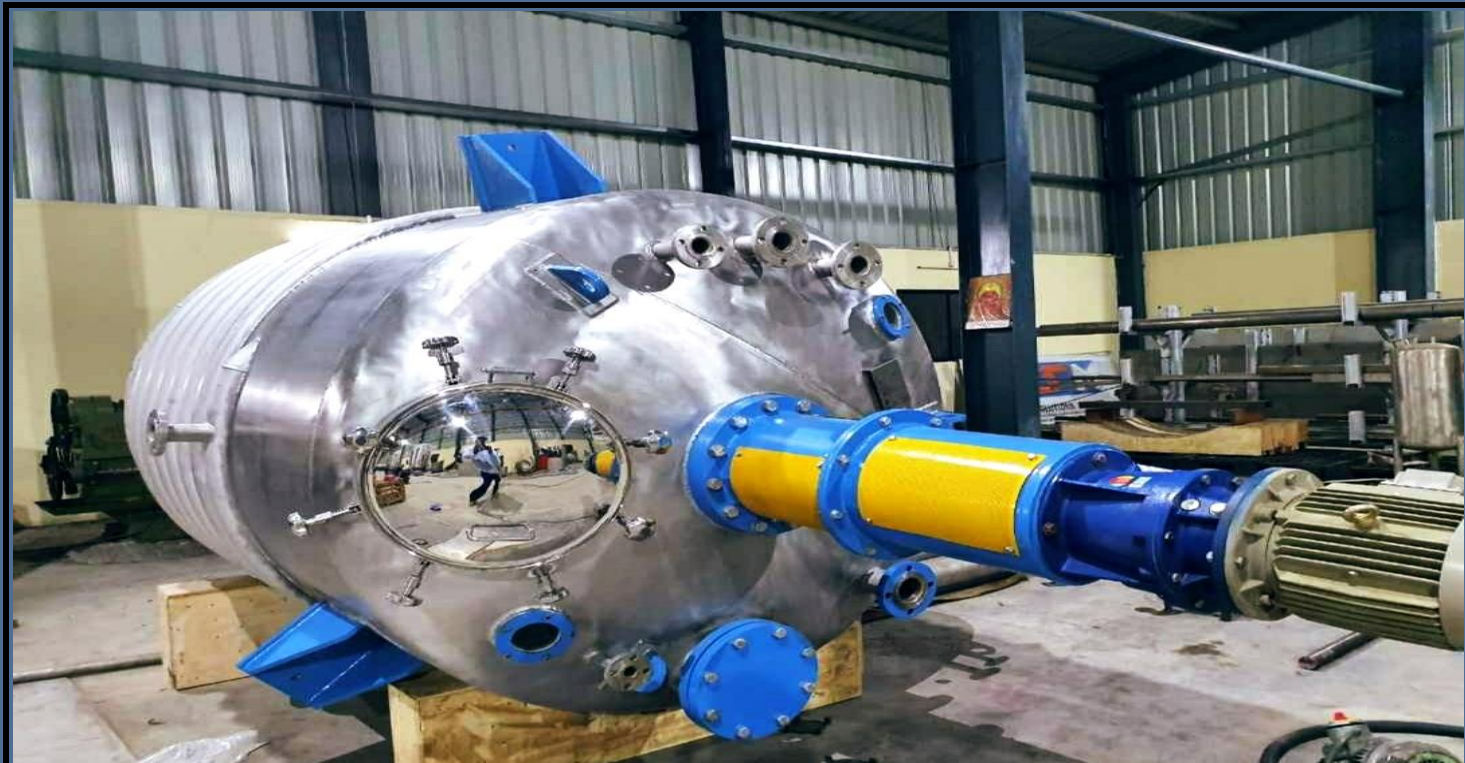
Limpet Coil Reactor with Agitator
