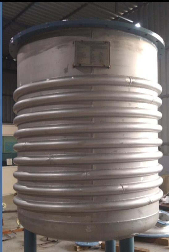
Reactor with Body flange & Limpet Coil
