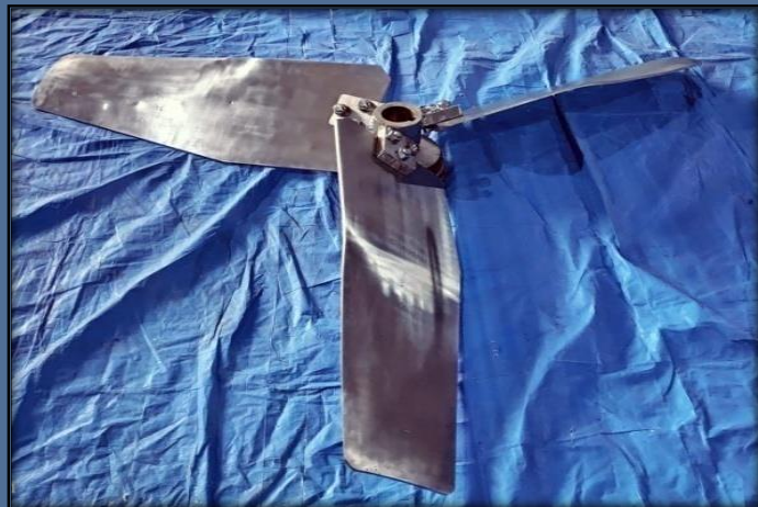
Hydrofoil Impeller (Ø2.0 mtr)
