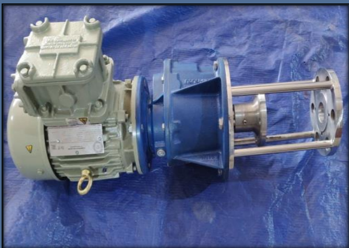
Anchor Agitator Assembly (Pharma Application)
