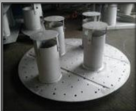
Pan Type Liquid Distributor
